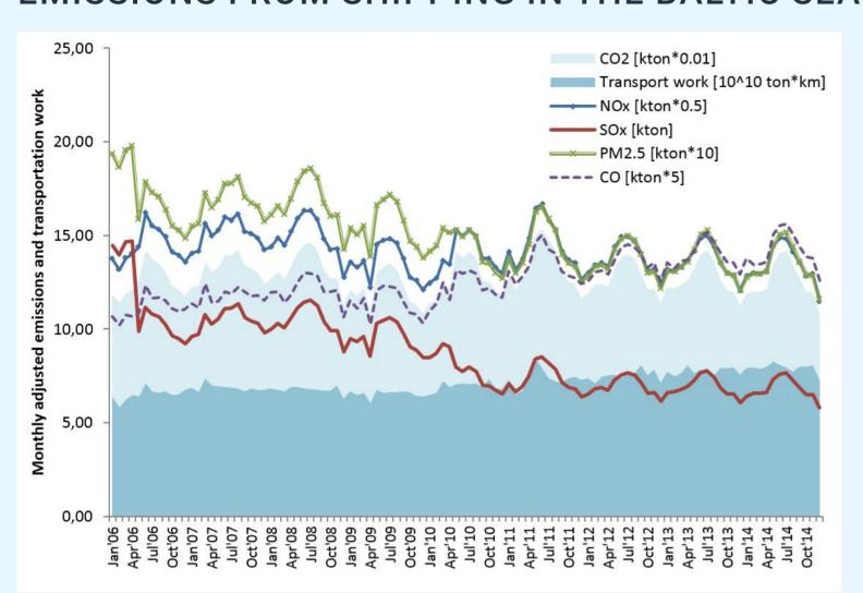
Improvements to the engines, better propeller performance and high-tech coatings, as well as friction-reducing air cushions and slow steaming might reduce carbon and sulphur emissions. Until now carbon emissions have stayed the same!
