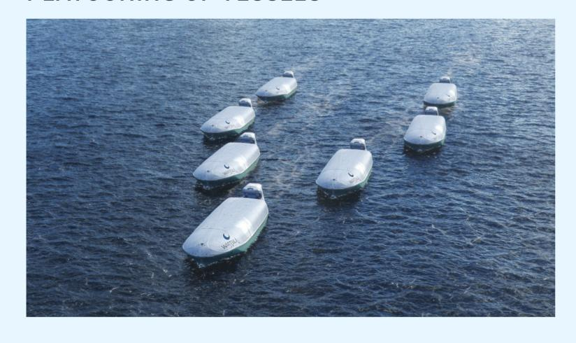
Trains of ships in which only the front ship is manned, while the others follow autonomously.
